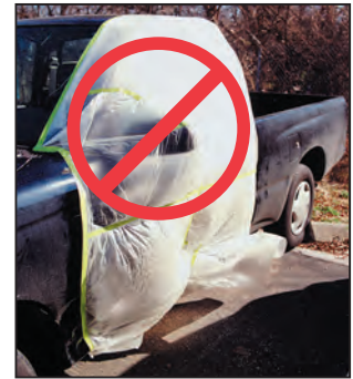
Eliminate jerry-rig attempts to cover crash damaged vehicles sitting outdoors awaiting repair.
