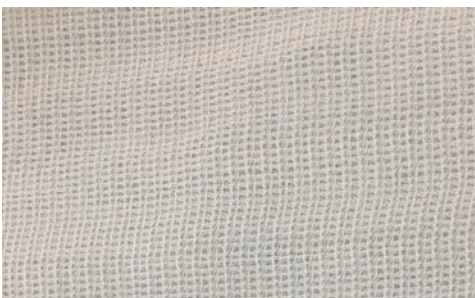
New Dirt Trap and Overspray Netting
