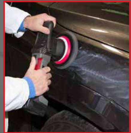
Excellent for removing scratches and minor defects. Produces a mirror gloss without holograms or wheel marks
