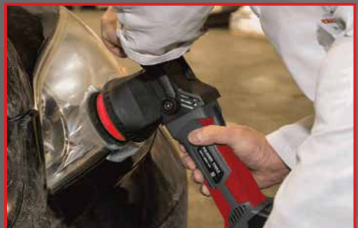
Polished with 3.5" Dual Density Pad and 1- Step Polish
